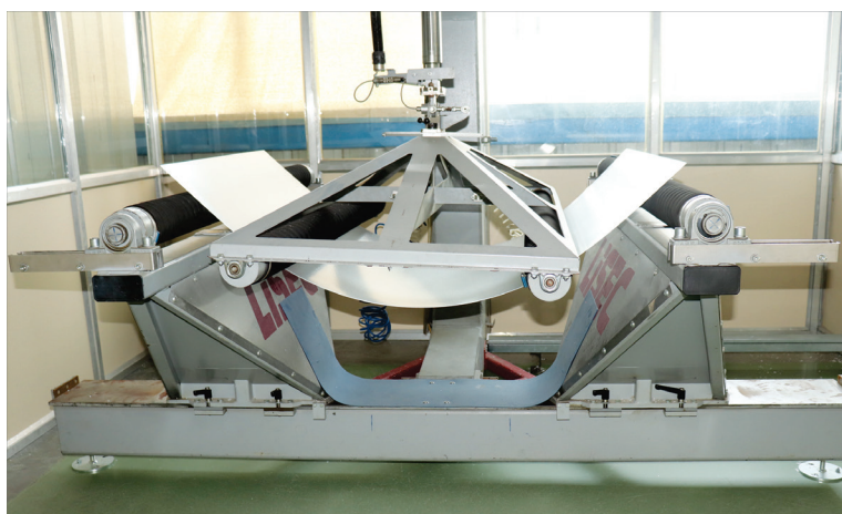
Performing a bending test on 2mm solar glass.
